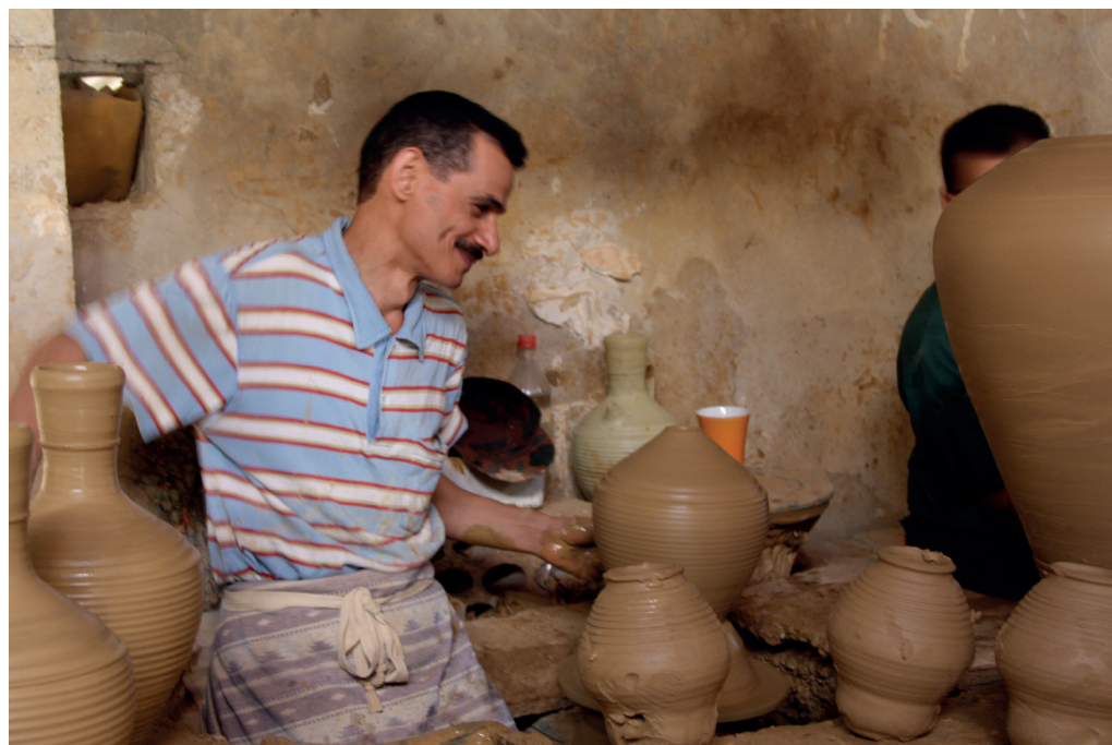
Figure 3 – Zizia potter sitting at his wheel with pots in three stages of work. In front of him, within reach, stand three incomplete pots, bases facing upwards. After they dry slightly, each will be placed upside-down on the wheel for further work. Each has a finished ring base above a thick lump of unworked clay. The potter will shape the pot upper body from the thick reservoir of wet clay attached to the finished base, as he has done for the piece still in progress on the wheel. Two pots on the left show the full shape (photo by Stefanie Elkins).
